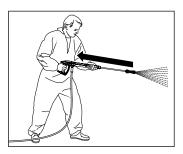
When using high-pressure water for cleaning, make sure that there is a clearly noticeable recoil effect on the lance. Therefore ensure a firm footing (see technical data).
