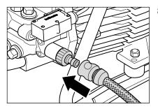
8. Connect water hose to water inlet (minimum requirements; 5 m hose length, cross-section ¾", 10 bar). The high-pressure cleaner may be connected to a water mains (1-10 bar pre-pressure) with either cold or hot water (up to 60 °C). The K 1622 TS provides the opportunity of sucking in water out of a container (see direct suction).
