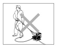
Never direct the high-pressure jet at the highpressure cleaner itself! The high-pressure cleaner may not be placed within reach of the highpressure jet spray mist!
