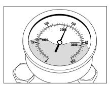
Having closed the trigger gun with safety catch, the high-pressure cleaner must shut down and the stainless steel pressure gauge must show "0" bar. If not shut down and the stainless steel pressure gauge continuously shows full pressure, this could be due to leakage at the high-pressure pump, at the pressure switch, at the high-pressure hose or at the trigger gun with safety catch.
