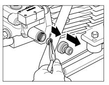
Check water inlet filter for cleanliness prior to putting the high-pressure cleaner into operation.
