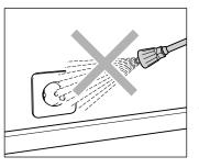
Never direct the high-pressure jet at power sockets or any other electrical installations! Within the working area, all live parts are to be protected from both water jet and spray mist.
